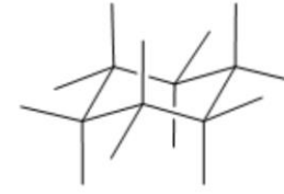
typical drawing showing all the axial and equatorial positions. Each C looks tetrahedral
